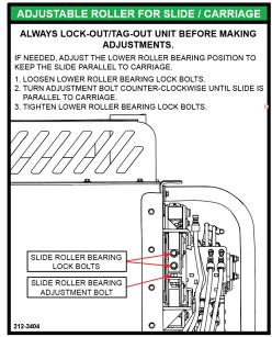
Figure: Adjustable Roller for Slide / Carriage, 212-3404
