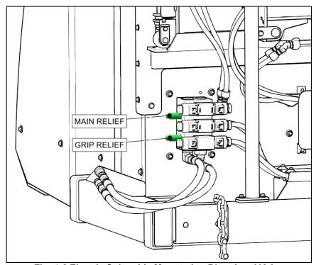
Fig. 4-6 Electric Solenoids Mounted to Directional Valve
