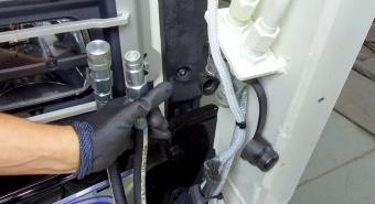
7. Disconnect the two Packard electrical connectors and the Curotto-Can® work lights harness connector (if equipped). Remove any cable ties securing the electrical cables to the truck-side. See images below.
