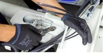
9. Un-route the electrical cables and hydraulic hoses from underneath the routing guide bar. Then connect the Curotto-Can® pressure and return lines together to help keep them clean. See image below.
