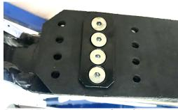
Belt Bolted Through Middle Set of Holes on Belt and Bracket
