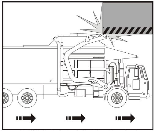
Fig. 3-1 Positioning the Curotto-Can for long distance travel
