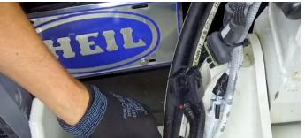
8. Disconnect the two Curotto-Can® Auto Cover air lines (if equipped). See images below.
