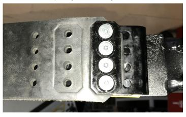
The grabber belt bracket has 3-hole positions on 1/2" spacings. See the figure below.
