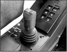
Fig. 3-15 Curotto-Can electric joystick
