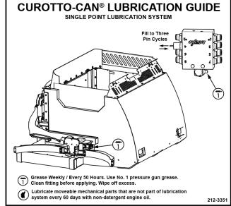
Figure: Curotto-Can Optional Single Point Lubrication Guide, 212-3351
