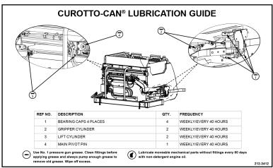
Figure: Lubrication Guide, 212-3412
