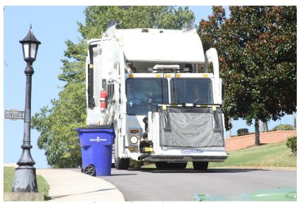
Fig. 3-3 Curotto-Can in Collection Position
