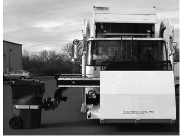
Fig. 3-6 96 Gal. Cart Engagement When the Fork Pivot Tube is at the 9" (23cm) Working Height
