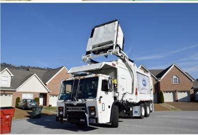
Step 3. Use the fork retract function to invert the Curotto-Can® and dump the contents
