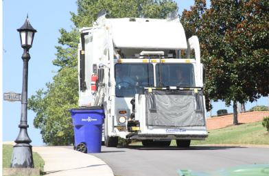
Step 2. Raise the Curotto-Can<sup>®</sup> using the arms up function only until it is in the position shown - arms against the bumper
