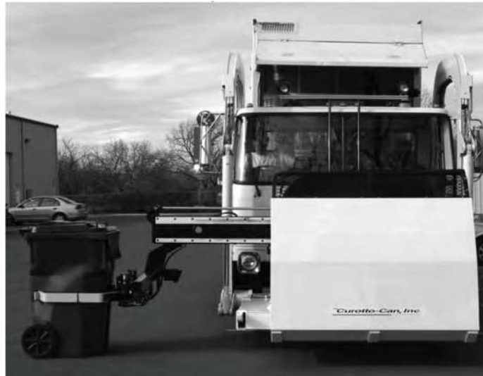
Fig. 3-6 96 Gal. Cart Engagement When the Fork Pivot Tube is at the 9" (23cm) Working Height
