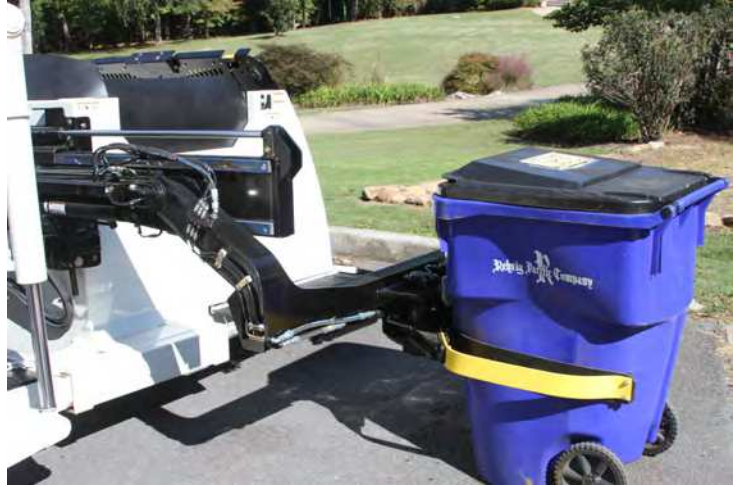
Fig. 3-12 Maximum Arm Extension is 60"
