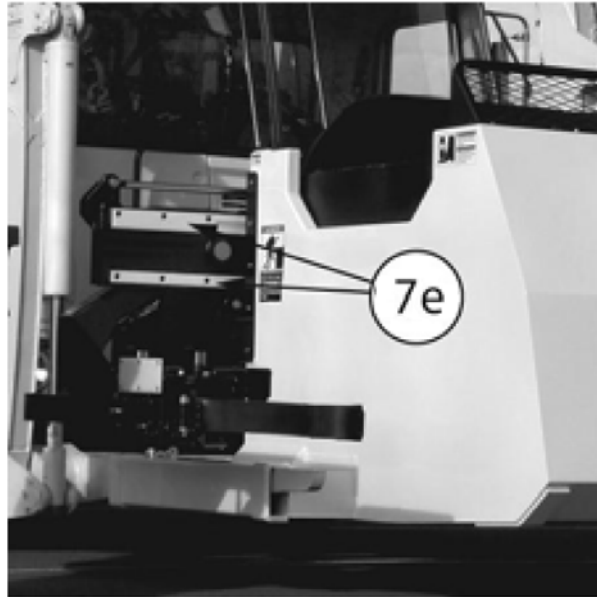
Fig. 3-44 Mechanical on Curotto-Can Assemblies Weekly Check Slide Assembly Nylon Wear Strips
